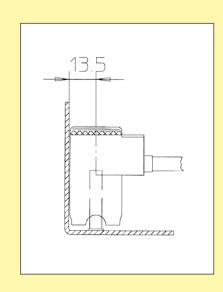
MINIMUM DISTANCE FROM STUD CENTRE TO INSIDE FACE OF VERTICAL WALL IS 13.5mm
