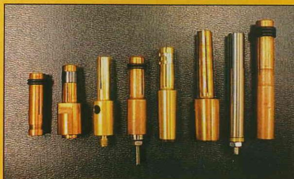
**NOSE CONE ASSEMBLIES:** are used to accurately locate studs when using templates. These are available in 3 diameters: 30mm (standard), 1" and 22mm. Nose cones can be cut to fit around complex shapes or manufactured with extended "chimney" to locate inside high sided narrow components such as deep channels or to totally enclose the weld area for noise reduction.
