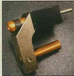
This assembly must be insulated. The insulation prevents equipment shut-down should the assembly touch the end-cap. Insulation must be checked regularly and replaced if there are signs of wear.
