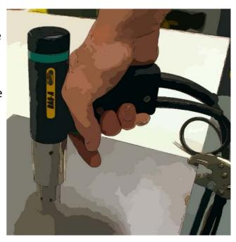
Once welding has taken place. Draw the pistol off the welded stud. Always lift the welding pistol vertically from the welded stud. Failure to do this may cause damage to the chuck, which will result in the chuck and stud arcing together during subsequent welds and thereby reducing the working life of the chuck.
