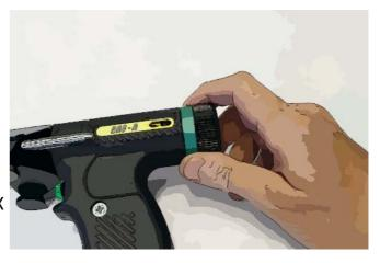
Stage two is to "zero" the lift. NOTE Ensure that the pistol is not connected to the
