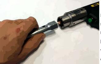
IMPORTANT! Do not over-tighten chucks. This requires only hand tightening. Over-tightening may result in un-warrantied damage to your pistol.
