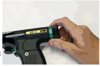
Stage two is to "zero" the lift. NOTE Ensure that the pistol is not connected to the controller whilst performing this stage. To do this
