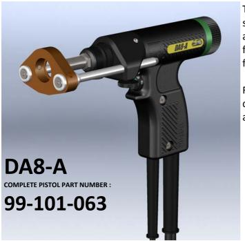
The basic standard model of the DA8-A pistol is shown here on the left. This model is supplied rigged as standard to use European screw-on chucks and for welding standard drawn arc studs with ceramic ferrules.
